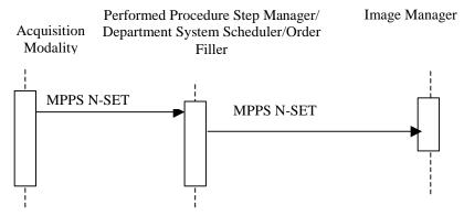
Note: The diagram above shows the sequencing of messages for the Modality Performed Procedure Step SOP Class. Acquisition Modalities will also implement the Storage and Storage Commitment classes. The timing relationship between PPS messages and Storage and Storage Commitment messages is not specified. That is, PPS messages may occur before or after storage requests.
