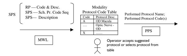
Upon obtaining a MWL from the Department System Scheduler/Order Filler the Acquisition Modality is required to display the attributes Scheduled Protocol Code Sequence and Scheduled Procedure Step Description (this requirement is part of Rad–5 and EYECARE-1].
