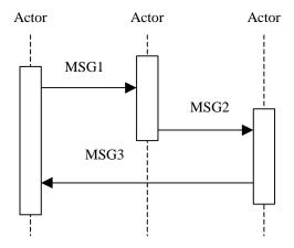
The interaction diagrams used in the IHE Technical Framework are modeled after those described in Grady Booch, James Rumbaugh, and Ivar Jacobson, *The Unified Modeling Language User Guide*, ISBN 0-201-57168-4. Simple acknowledgment messages are omitted from the diagrams for brevity.
